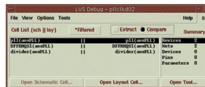
Figure 3: GUI-guided LVS debug environment helps locate and fix the layout easily
